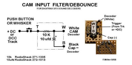
Note that the Triggering voltage can be from either DCC track circuits, if the SFX Sound Decoder is powered by the DCC track, or from a +DC voltage source if the Decoder is powered by DC rather than DCC. Connections are made to the Decoder CAM line (white wire on speaker side of decoder) and the black lead going to the Decoder external capacitor. (This is actually the Decoder ground.)
