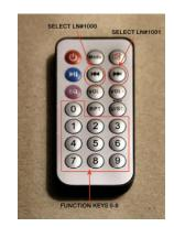
*LocoNet* library developed by Alex Shepherd to send LocoNet commands, and the Arduino library *IRremote* to help decipher the IR commands. I used the IR Pad shown since I had a bunch of them from previous projects, but almost any IR remote, including TV remotes, could be used after determining the codes they produce.
