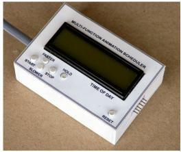
The time of day is presented on an LCD with custom enlarged numerals with a time of 01:00 AM to 12:59 PM. The in-memory script actually uses a 24 hour format (01:00 to 24:00) converted for display.
